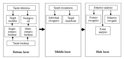
Fig. 2. Intelligent video monitoring algorithm flow
